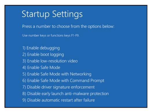
Driver verification will be dsiabled only until the next reboot (it will be enabled automatically again when the computer starts nex time). Please connect your jBotBrain board into the USB port and select corret path to the drivers when asked by the operating system.
